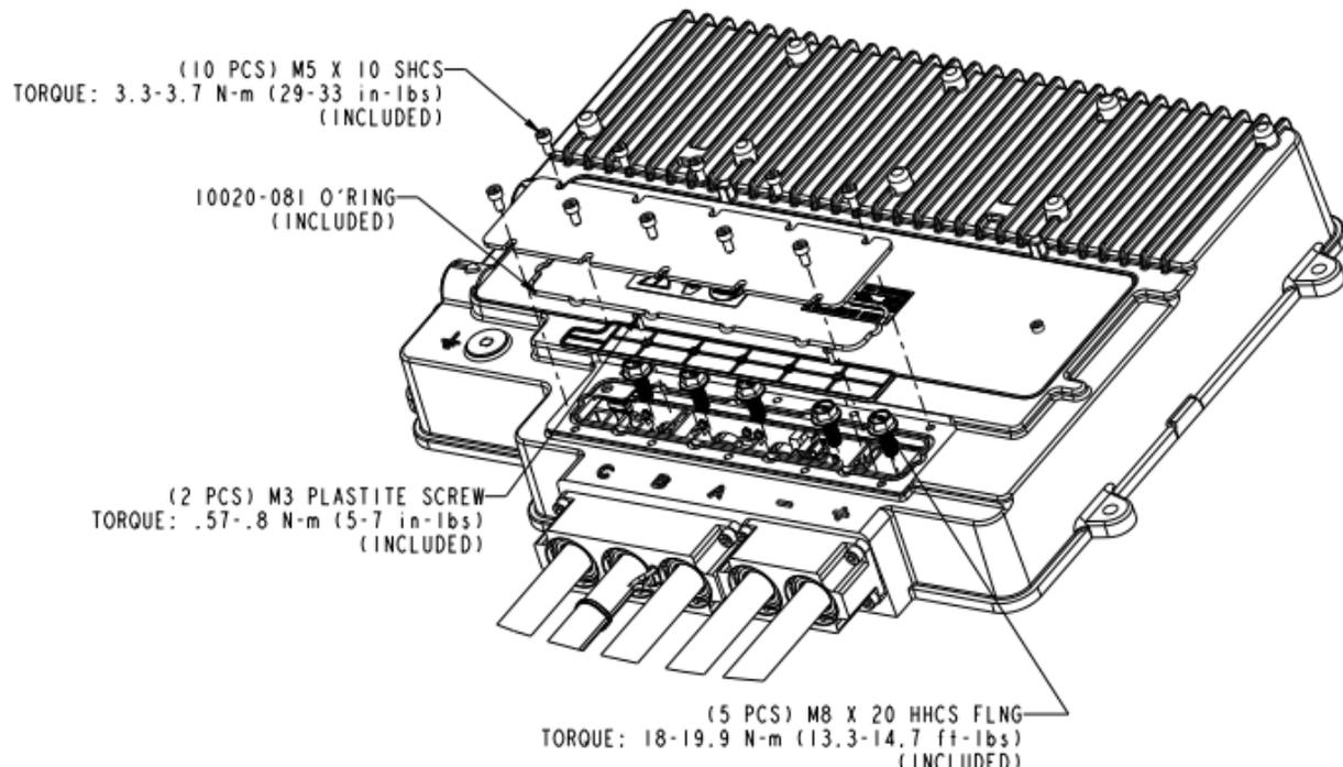
Figure 3.4 Exploded View of the Controller Connections
