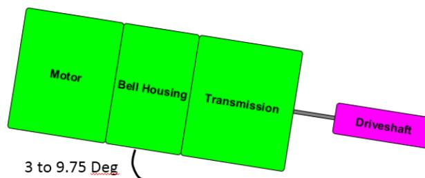
Figure 2.4: Mounting angle limits
