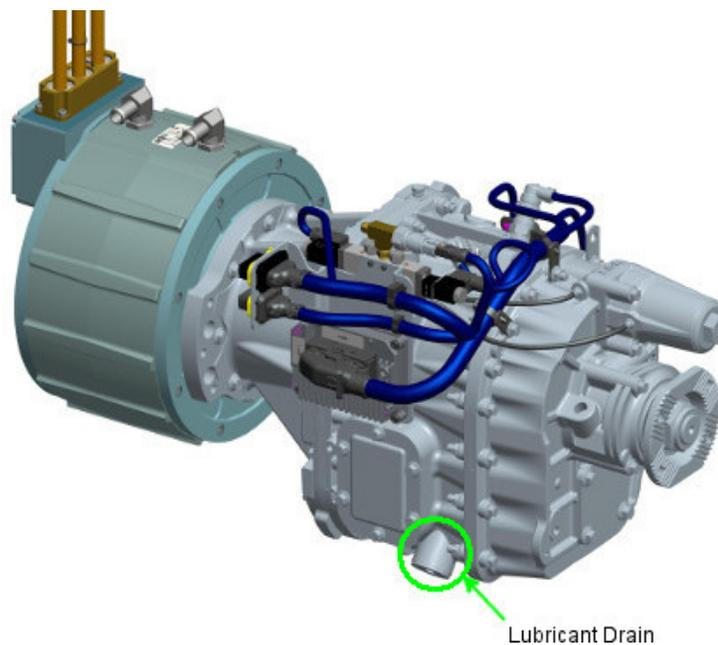
Figure 2.9: Lubricant Drain Port
