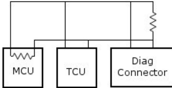
Figure 3.13: TCU to MCU CAN bus
