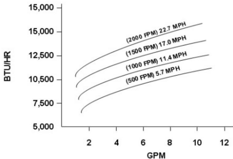
Figure 2.11: Eaton 18025 cooler heat transfer based on 38° C (100° F) temperature differential
