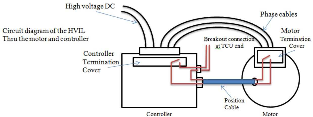
Figure 3.3: HVIL daisy chain routing through the controller and motor
