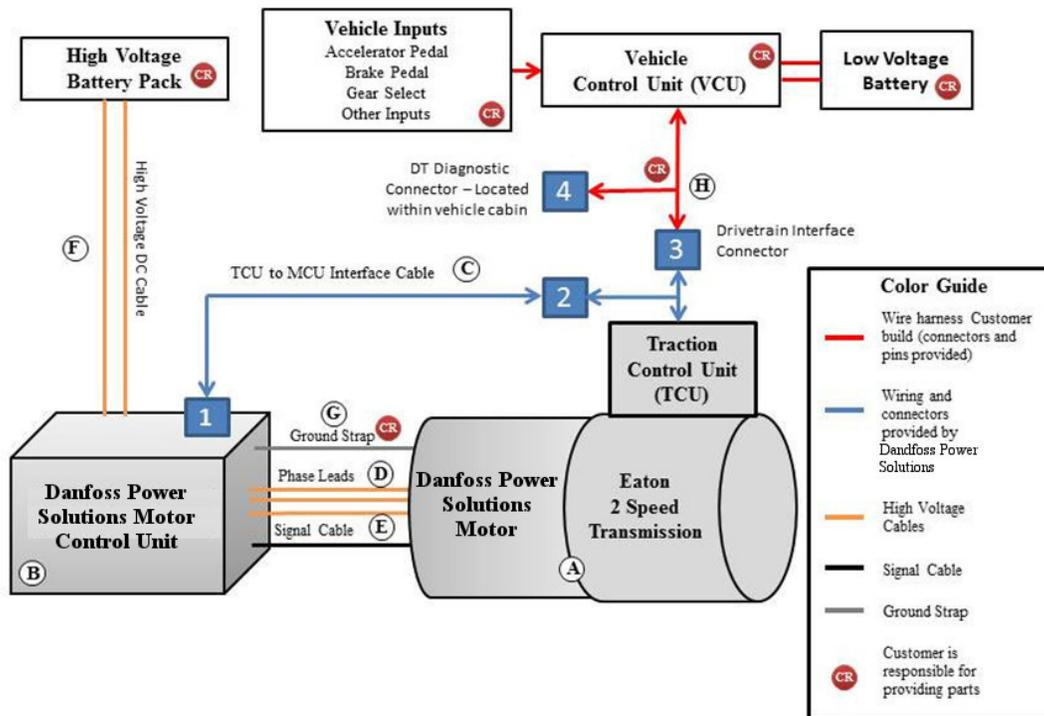
Figure 1.1: Block Diagram of the Total System
