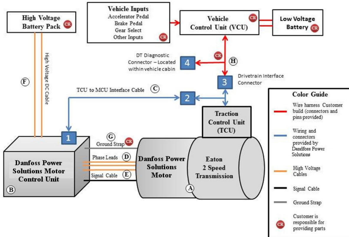
Figure 5.1: Block Diagram of Electric Vehicle Drive System
