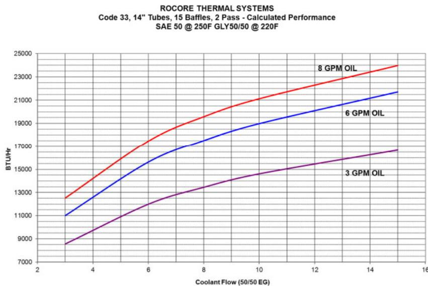
Figure 2.13: Eaton 5586750 heat exchanger heat transfer
