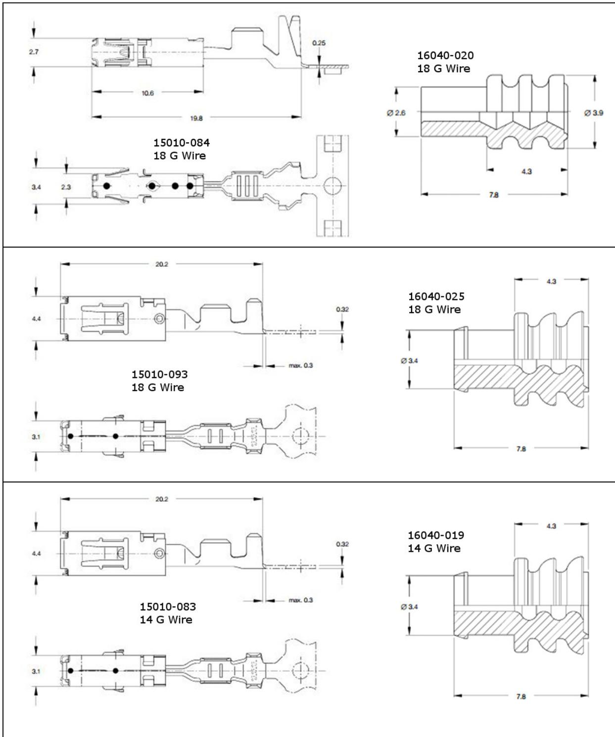
Figure 3.11: Drivetrain Interface Connector terminals and wire seals
