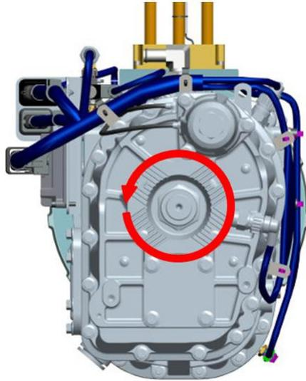
Figure 2.5: Direction of rotation in forward
