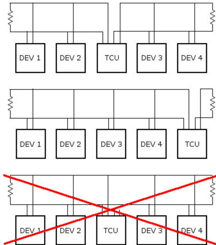
Figure 3.12: Allowed VCU to TCU CAN Bus Configurations
