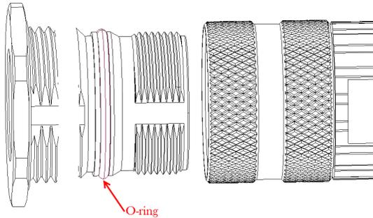
Figure 3.5: Signal Cable Connection – Insertion
