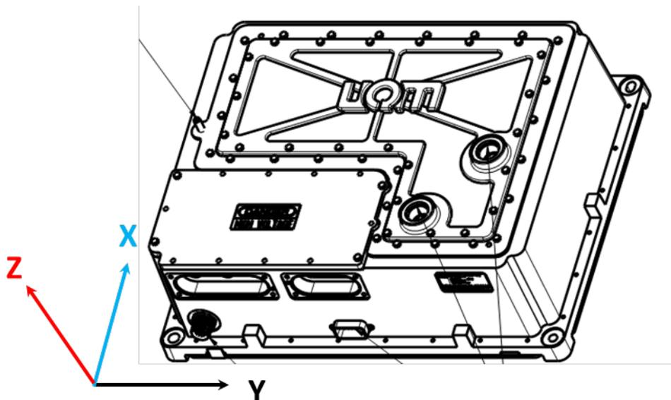
Figure 9.1: Controller Axis Orientation
