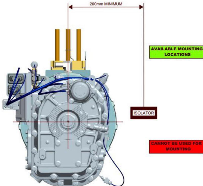
Figure 2.3: Approved location of vibration isolators.
