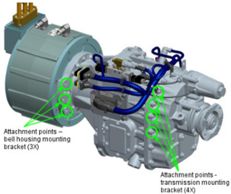
Figure 2.2: Right Side – attachment points for bell housing & transmission mounting brackets.
