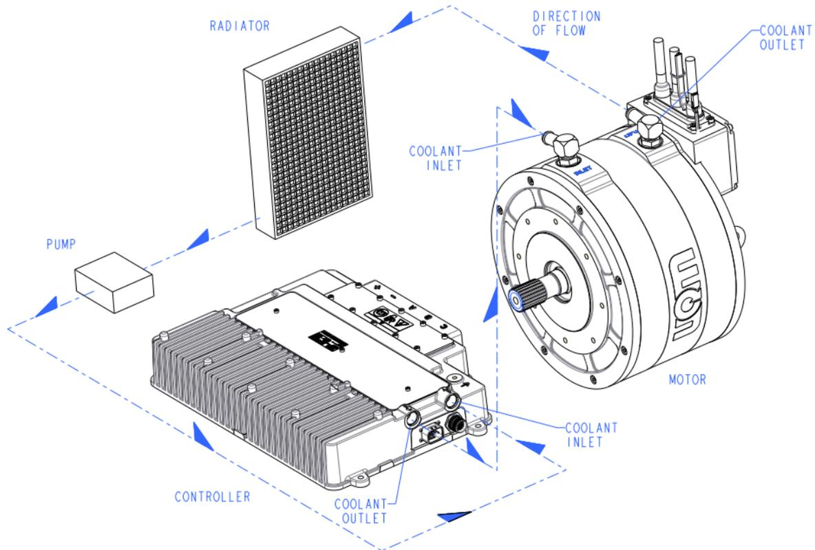
Figure 4.1: Recommended Liquid Cooling Setup
