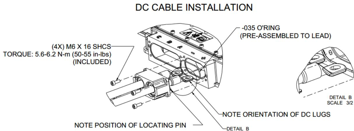
Figure 3.2: Controller Connections
