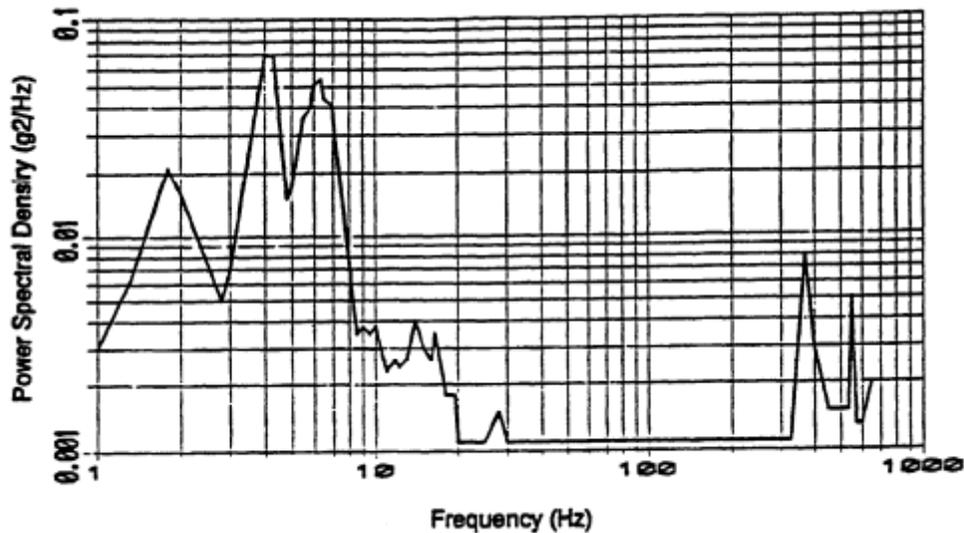
Figure 9.2: SAE J1455 PSD Bobtail vertical Mid frame, Heavy-duty Truck Profile
