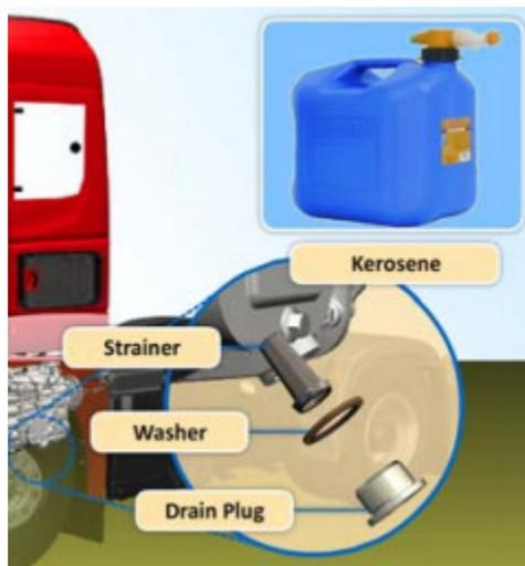
Figure 2.7: Transmission lubricant drain
