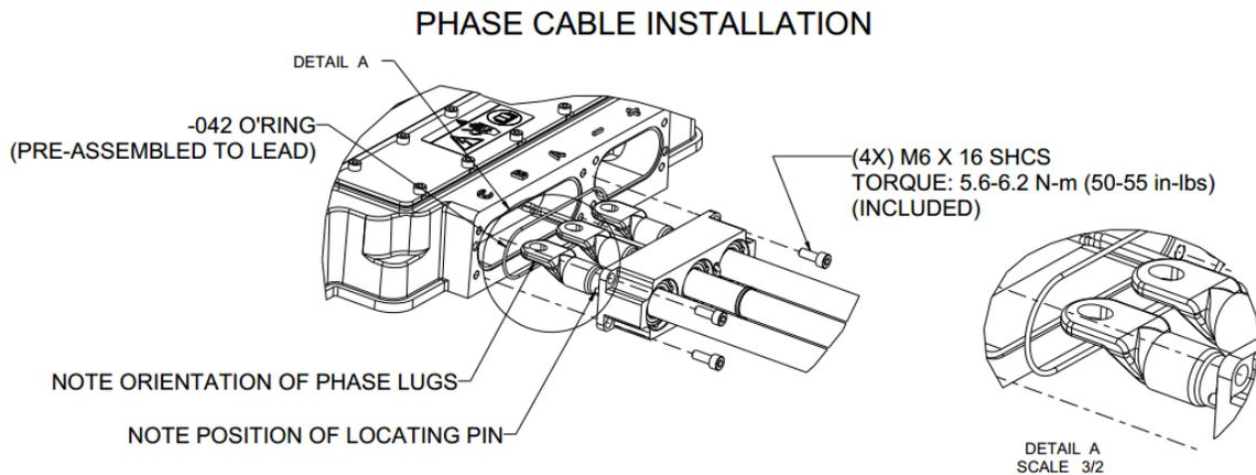
Figure 3.1: Controller Phase Connection
