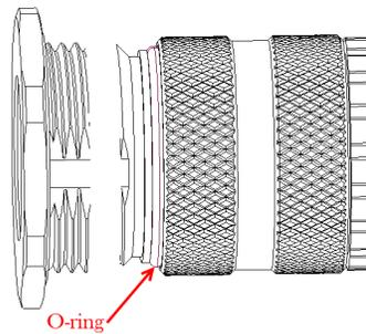
Figure 3.6: Signal Cable Connection – Tightening
