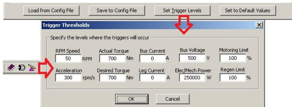
Figure 8.20: DAQ Trigger Thresholds
