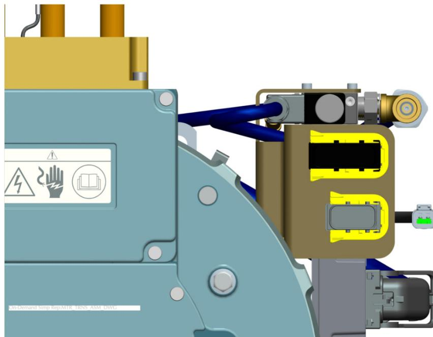
Figure 3.8: Connector Bracket
