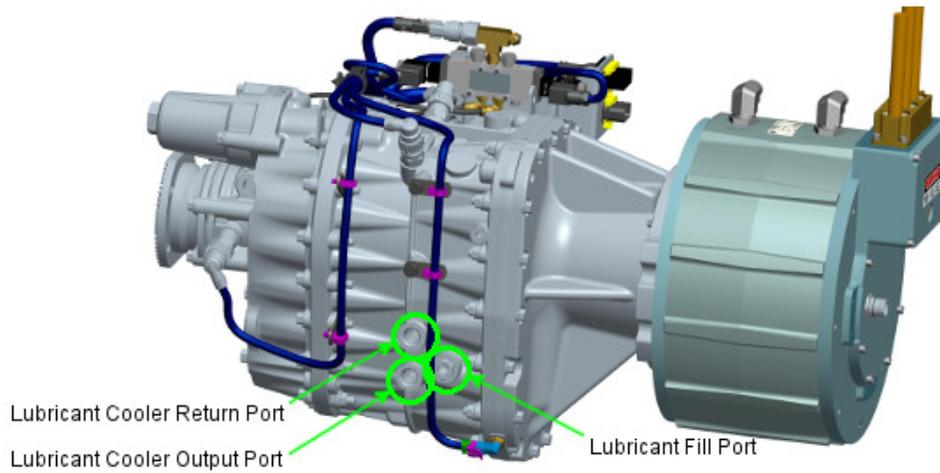
Figure 2.8: Eaton Transmission Lubricant Ports
