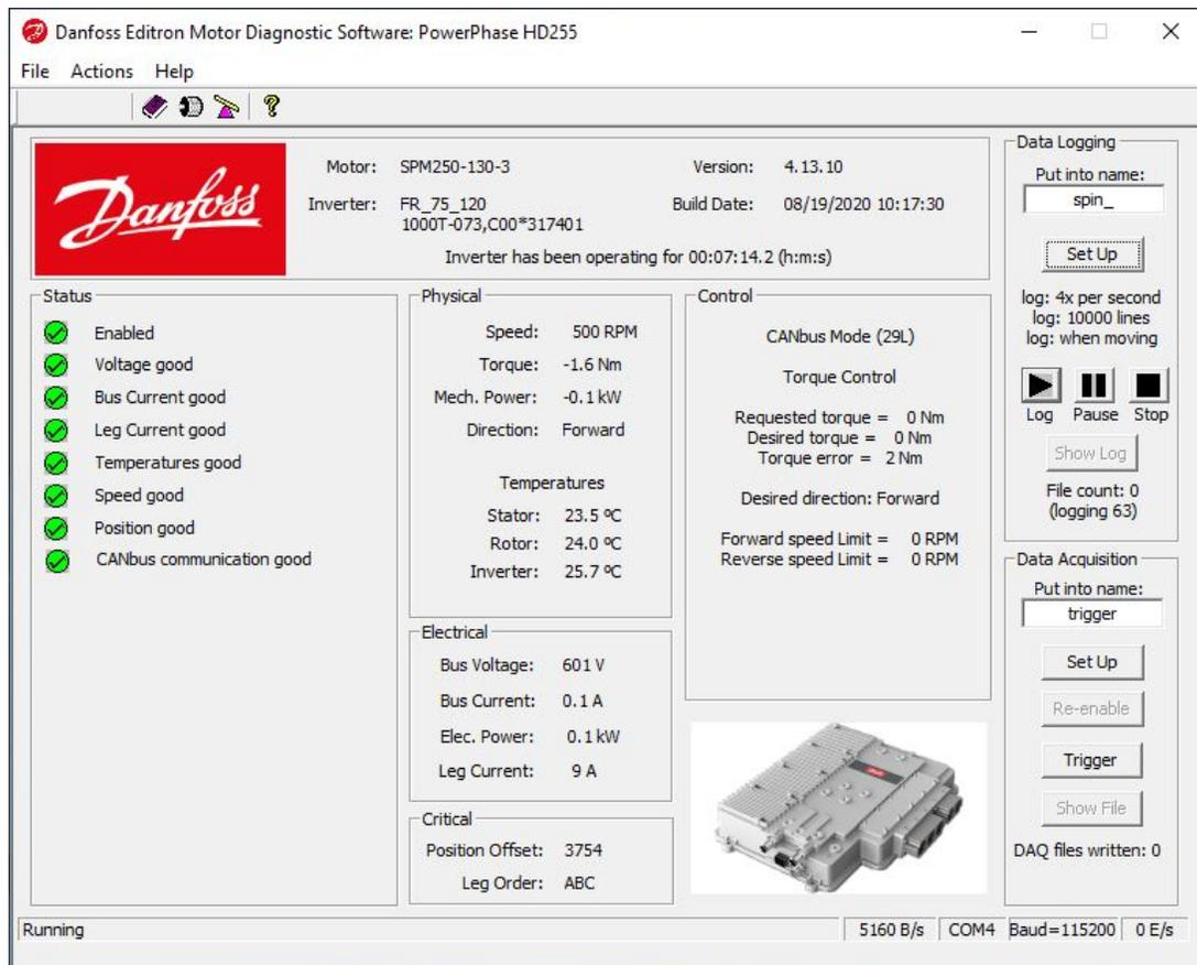
Figure 8.1: Danfoss Power Solutions Motor Diagnostic Software Front Panel
